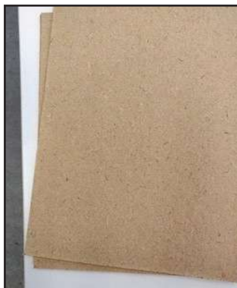
Panel Board prepared by ECOR Panels, The Netherland using rice straw Chemical and Chemi-thermo mechanical pulp produced by CPPRI
