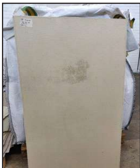
Panel Board prepared by ECOR Panels, The Netherland using rice straw Chemical and Chemi-thermo mechanical pulp produced by CPPRI
