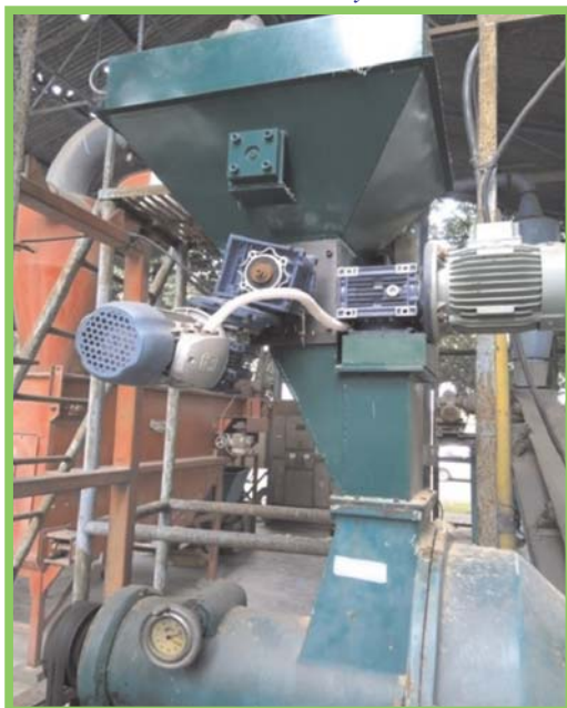
Feeding System of Bagasse Depithing Pilot Plant
